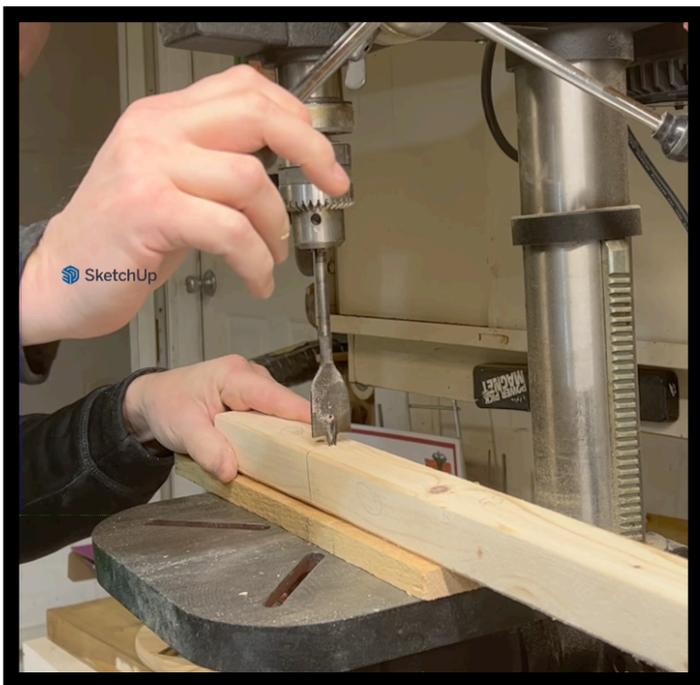
Place a 1" wood boring bit into chuck and tighten. Be sure to use a scrap piece of wood under the legs to prevent tear-out and protect your table.
