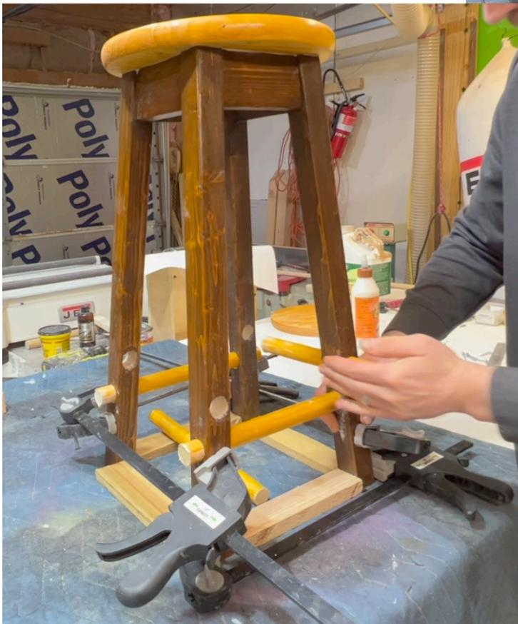
TIP: For accuracy I put blocks and clamps on the legs prior to inserting the dowels. This is optional, but I recommend it just in case you have to hammer/bang dowel and you won't have to risk breaking the legs. Plus it might help true-up some of your work. Leave blocks and clamps on overnight while glue dries.
